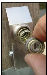
The self-aligning bearing assembly of the soon to be launched commercial version of the Oscillot system
